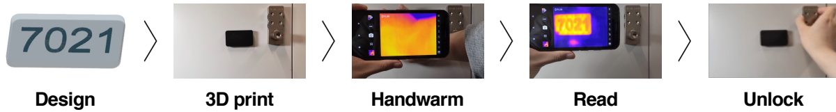
Fig. 23. Example of hidden PIN code. Design: Four digits as the PIN code are embedded under the plate. Read: The PIN code is revealed under a thermal smartphone after hand-warming the 3D printed plate. Use case: In an escape room, players are required to find the hidden PIN code for the locker to acquire necessary items.
