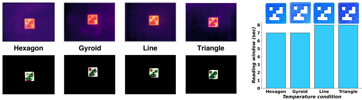
Fig. 10. Illustration of thermal imaging with different infill patterns. The reading succeeded with all four infill patterns. The figure on the right shows the reading window for infill pattern tests.
